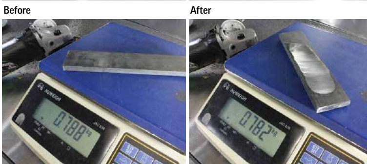
Stock removal testing of flap discs
